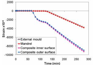
Fig. 6 Strain evolution at the interfaces.
