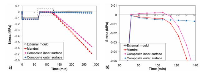
Fig. 7 Stress evolution at the interfaces: a) during the whole cure cycle; b) at the end of the isotherm.
