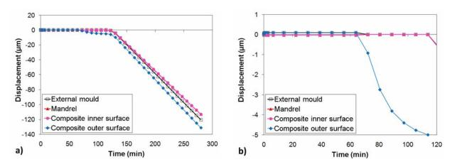
Fig. 8 Displacement evolution at the interfaces: a) during the whole cure cycle; b) during the isotherm.
