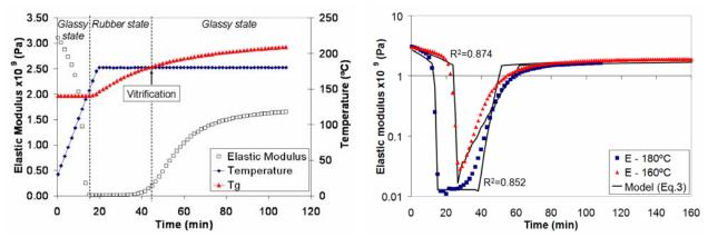
Fig. 2 Evolution of the elastic modulus with temperature and time.
