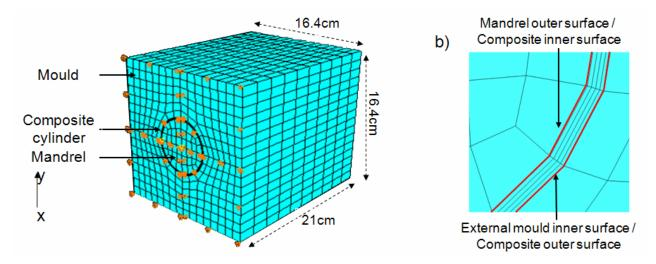
Fig. 4 a) Finite element geometry of the composite cylinder in the mould and symmetric boundary conditions – b) Details of the composite cylinder through thickness mesh.
